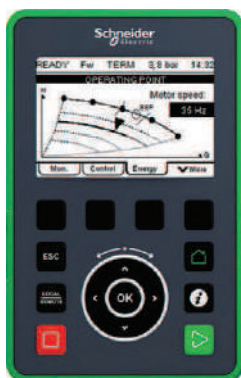
Remote graphic display terminal (example shows dynamic pump operation in relation to its optimum operation)
